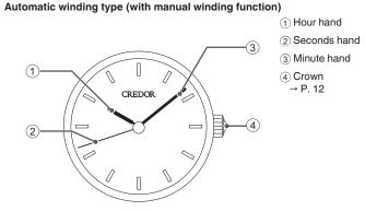
How to wind the mainspring  $\rightarrow$  P. 13 How to use (For models with a seconds hand or a small seconds hand)→ P. 15
