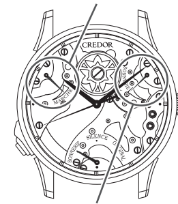
Power reserve indicator for the hour striking function
